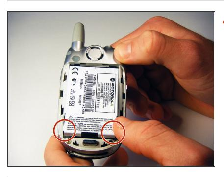
Lever the battery out by pressing upwards on the bottom corners of the battery.
