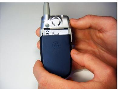
Press down on the chrome button on the bottom of the chassis. Simultaneously slide the back cover down, away from the phone.
