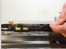
Detach the three different connectors located on the back of the screen.
