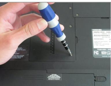
Unscrew the three 4.6 mm screws holding the panel using a #1 size Phillips head screwdriver. The panel is centered on the bottom of the laptop.
