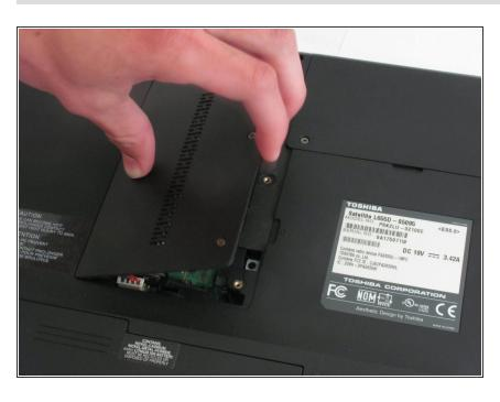
Remove the panel, firmly lifting from the indent. It is recommended that you leave the screws in the panel.
