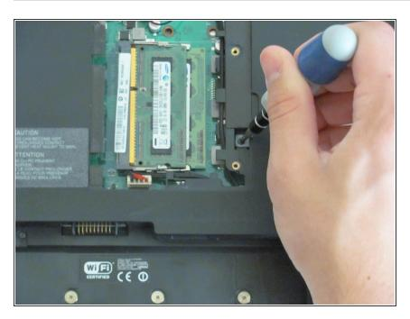
Unscrew the 3.9 mm screw located at the bottom right of the panel.
