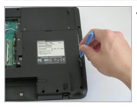
Use a plastic opening tool to pry the CD drive out of the casing.
