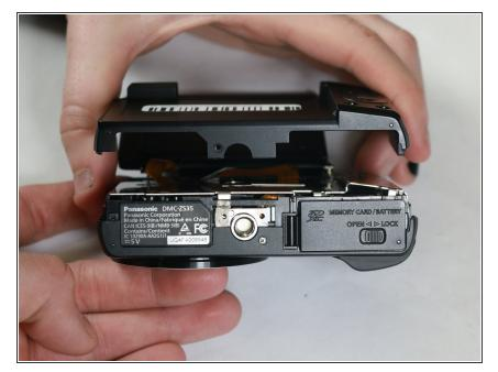
Gently pry apart the back casing from the body of the camera. It's recommended to apply as minimal force as is necessary to prevent unintended damage to the camera or the casing.
