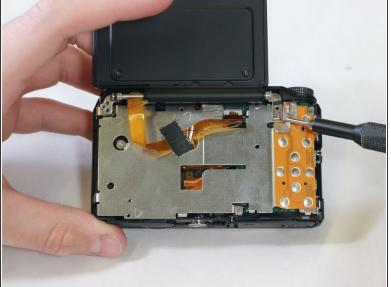
Unscrew the four 3mm screws holding the LCD screen hinge in place using a Phillips #000 screwdriver.
