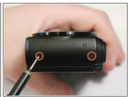
Remove the six 4mm screws located on the side and bottom of the camera casing using a Phillips #000 screwdriver.
