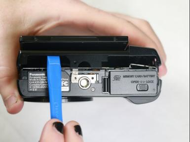
Use a plastic opening tool to carefully separate the back casing from the main body of the camera.
