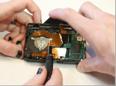
Remove the 2mm screws holding the lens in place with a Phillips #000 screwdriver, located along the perimeter of the lens component within its housing.
