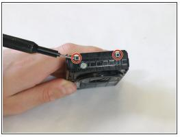
Remove the four 2mm Phillips #000 screws on the sides of the exposed internal metal plate within the camera.
