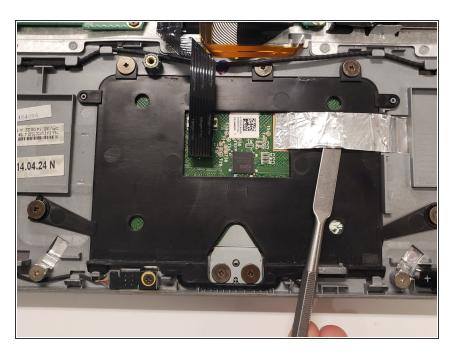
Use a spudger to remove the aluminum foil tape from the touchpad.
