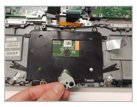
Use the pointed end of a spudger to remove the small triangular metal piece.
