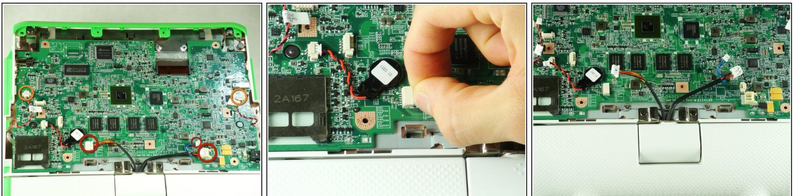
**⚠** Pull the connectors out by holding the plastic tabs and not the wires.
