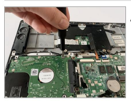
Remove the four Phillips #0 screws from the hard drive.
