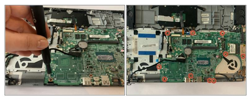
• Remove the ten Phillips #0 screws that attach the motherboard to the keyboard.
