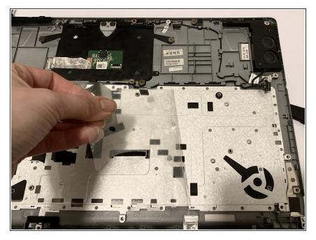
• Pull the clear plastic sheet from the top of the metal upper part of the keyboard.
