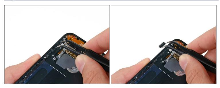
• Use tweezers to remove the volume-up button from the iPod.
