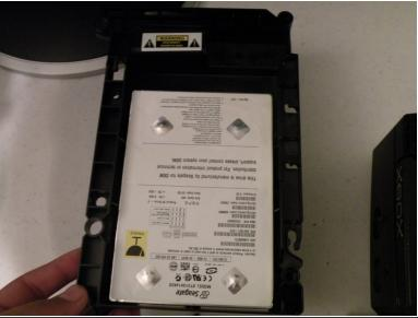
Lift the hard drive and the plastic attatched to it out, you will need to route the power cable so you can get it out.
