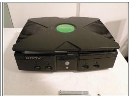
To remove the top half of the console, flip it upright and use a flathead screwdriver to separate the two halves.
