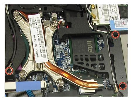
Remove the three (M2.5-8mm) "P" screws indicated to the left and place them in a labeled container.
