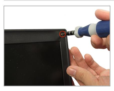
Using the Phillips #0 screwdriver, remove each of the six screws (M2.5-5mm) on the bezel and put them in a labeled container.
