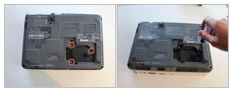
Remove three 11mm screws with a Phillips 2 screwdriver.
