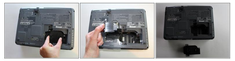
• Pinch on the two plastic clips and lift up to remove the bulb completely.
