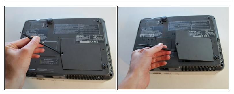
• Use a spudger to lift up the panel, then set it off to the side.
