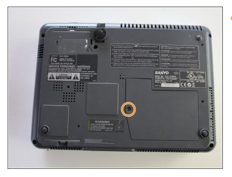
Remove one 9mm screw with a Phillips 2 screwdriver.
