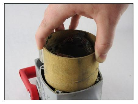
Lift the field out of the device, feeding the yellow wire through the handle.
