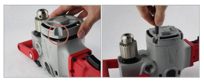
• Position the the drill upright and remove the four 19mm Torx T15 screws securing the motor cover.
