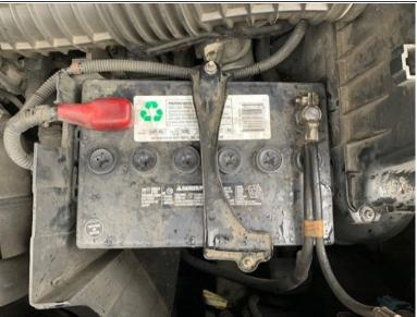
■ Take your new battery and place it where the old one was. Secure it into place with the plate, connect the negative (-) cable to battery. Then connect the positive (+) cable to battery.
