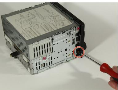
Using a Phillips #2 screwdriver, screw in both 5 mm screws on either side of the radio.
