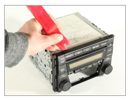
Using the spudger, pry the top control panel tabs off.
