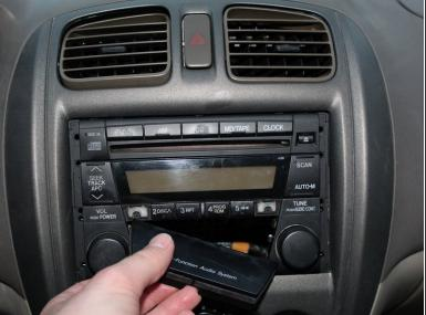
Use the spudger to remove this plastic cover to make the radio removal easier.
