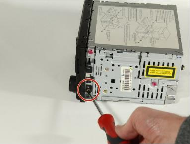
Using the Phillips #2 screwdriver, remove the two 5.0 mm screws on either side of the control panel.
