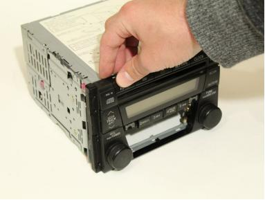
Re-clip the control panel back onto the radio.
