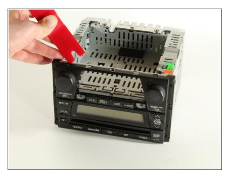
Using the spudger, pry the bottom control panel tabs off.
