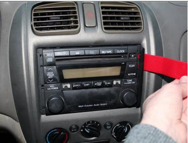
Use the spudger to remove both side covers to access the radio removal holes.
