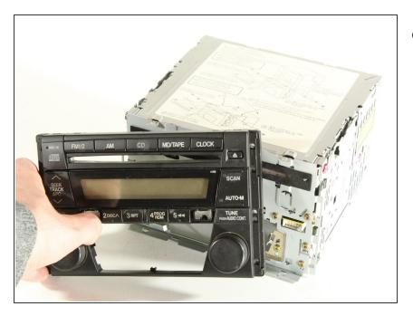
Remove the control panel.
