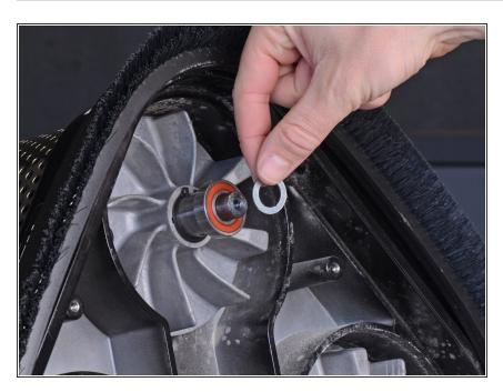
Remove the washer from the motor shaft.
