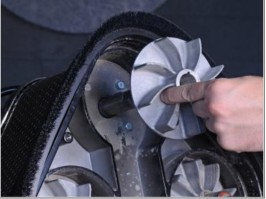
Slide the dust fan straight off of the motor shaft.
