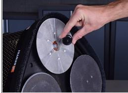
• Use a flathead screwdriver to pry off and remove the rubber plug in the center of the sanding disc.
