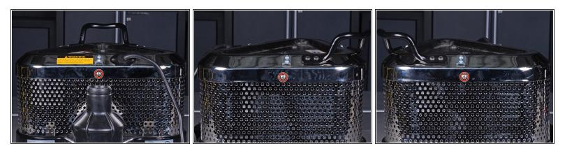
Use a Phillips #2 driver to remove three 22.1 mm-long screws securing the motor cover to the sander. There is one screw on each side of the sander.
