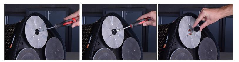
• Use a flathead screwdriver to pry off and remove the rubber plug in the center of the sanding disc.
