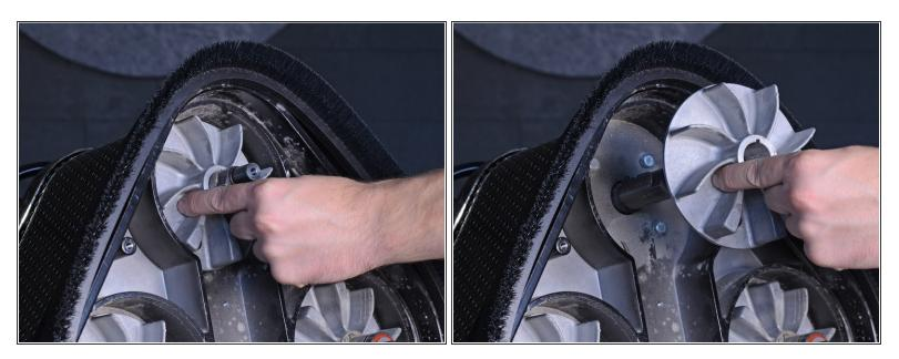
• Slide the dust fan straight off of the motor shaft.
