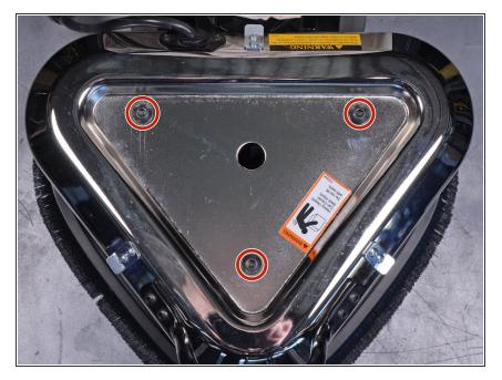
Use a 7/32" hex key to remove three 23.7 mm-long hex screws securing the motors to the motor cover.
