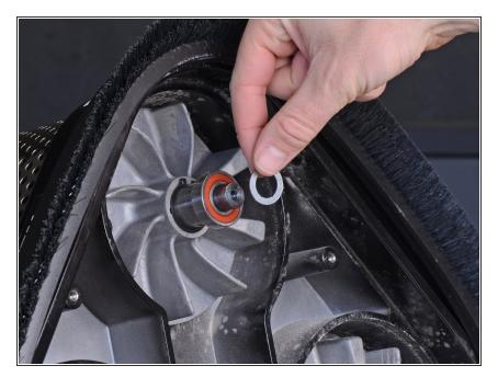
• Remove the washer from the motor shaft.
