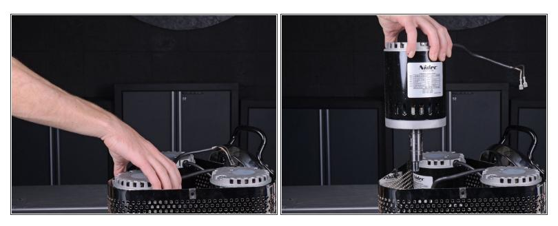
• Lift the motor straight up and remove it from the sander.
