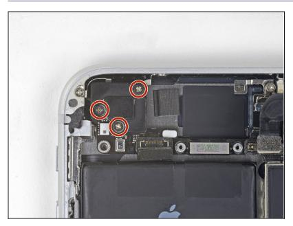
Remove the three Phillips 1.3 mm screws securing the top left antenna component.
