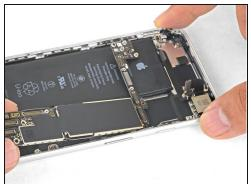
• Grasping it by the edges, lift the logic board near the battery connector and remove it.
