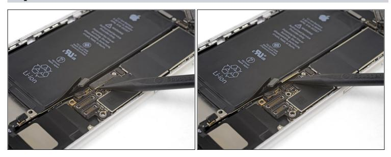
• Use the point of a spudger to pry up and disconnect the Lightning cable connector.
