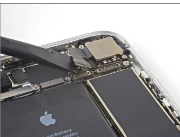
• Use the flat end of a spudger to disconnect the camera cable connector by prying it straight up from its socket.
