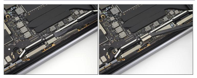
• Pry the display board flex cable straight up from its socket to disconnect it from the display board.
