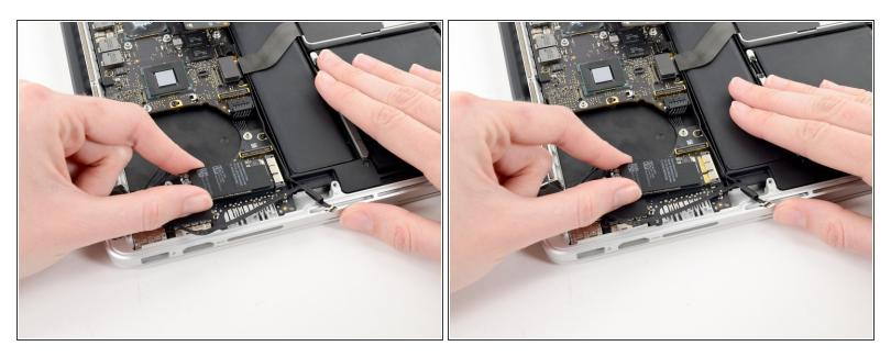
• Pull the AirPort board straight out of its socket on the I/O board.
