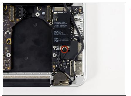
Remove the single 2.7 mm T5 Torx screw securing the AirPort board to the I/O board.
