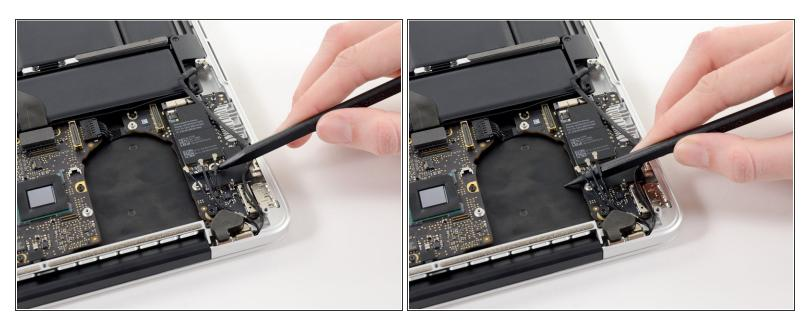
• Move the antenna cables aside, clear of the AirPort board.
