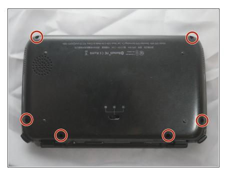
Remove the six PH #00 screws on the back of the GPD.
