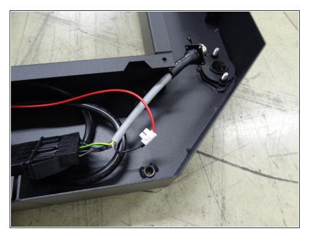
Attach the round connector coming from the door to the round plug in the roof
