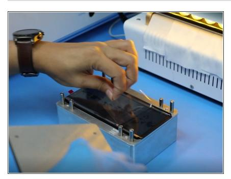
For this step, we can use an <u>easy</u> tape to tear off the protector of the touch screen.
