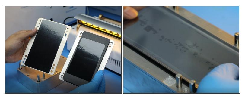
We put a new OCA on a new <u>Samsung Galaxy Note 8 touch screen</u>. It doesn't paste on the touch screen because the protector of the **OCA** is no need to be torn off. And you can move the <u>OCA</u> around until you get the right place.
