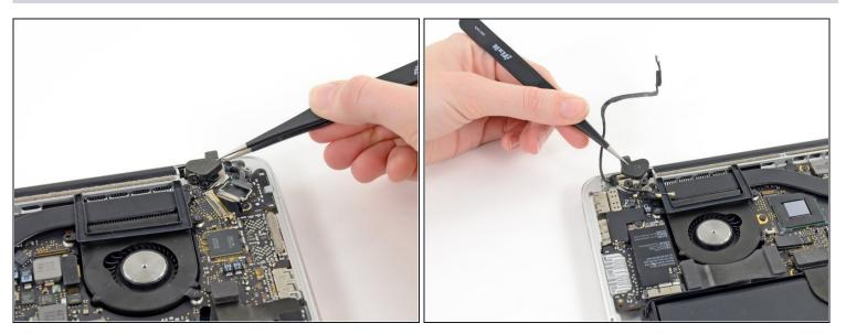
• Use a pair of <u>tweezers</u> to lift the rubber hinge covers up off the right and left display hinges.
