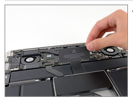
• Remove the plastic cover adhered to the battery contact board.
