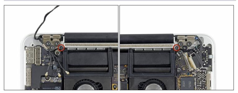
• Remove the two 3.1 mm T5 Torx screws securing the aluminum hinge brackets.
