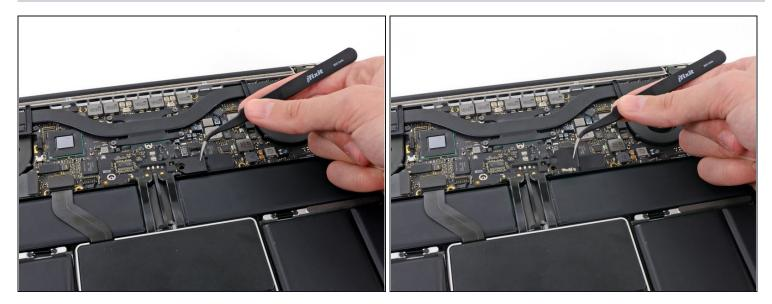
• Use <u>tweezers</u> to remove the small plastic cover located near the bottom right of the battery connector board.
