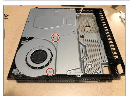
Use a Phillips #0 screwdriver to remove the two screws.
