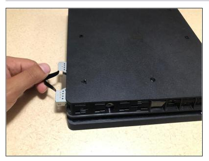
Pull the black ribbon on the side of the PS4 to remove the hard drive.
