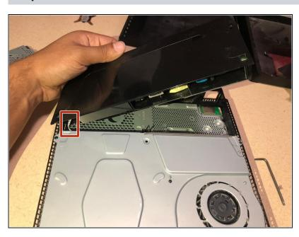
Remove the power supply completely by disconnecting the wire.
