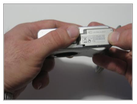
• Press down and slide the battery cover.
