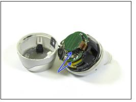
Since the Technics Headphone enclosure is glued together, the only way in was to cut into the headphone.
