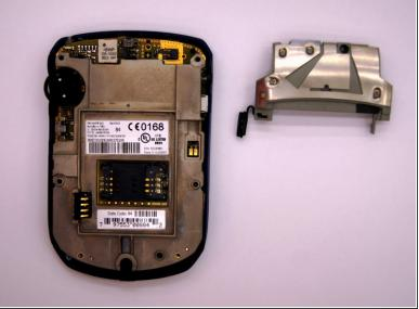
Using a Torx T6 screwdriver, remove the lone 1/8 inch screw that holds the upper metal bracket onto the larger metal bracket. Set aside the screw and the bracket.
