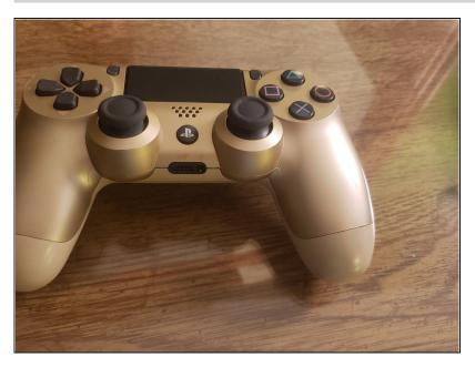
• Use a plastic spudger to open the case. Try not to scratch the plastic.
