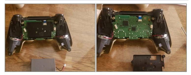
• Remove the battery and the screw underneath it.
