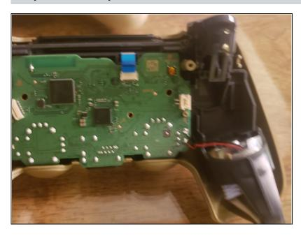
• The ribbon cable slots through the rectangular hole in the plastic beneath.
