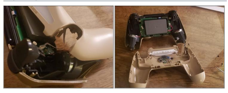
• Be careful opening the case because there is a ribbon cable holding the 3 halves together.
