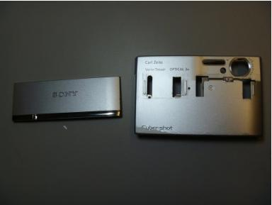
The front sliding lens cover is now removed and may be repair or replaced.
