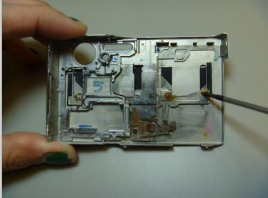
• Remove four screws using Phillips located on the inside of the front cover.
