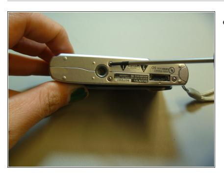
Use screwdriver to remove screws.
