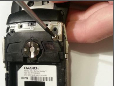
With the back cover removed, the antenna is now exposed. To remove it, take out the phillips screw holding it in place.
