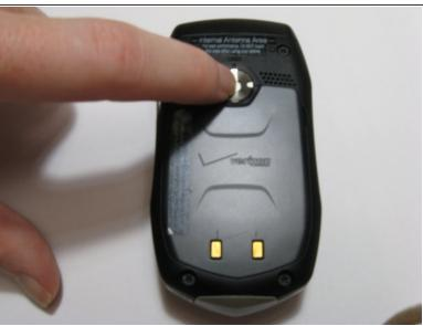
Turn locking device on back side of phone marked by the rectangle counter clockwise.
