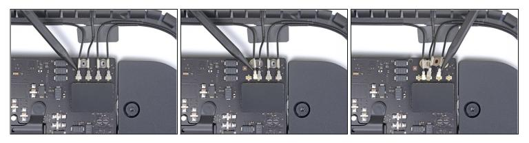
• Use the point of a spudger to pry all four antenna connectors straight up from their sockets and disconnect them from the AirPort/Bluetooth card.
