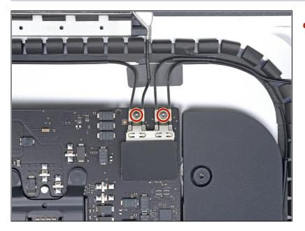
Remove the two 4.0 mm T5 Torx screws securing the four AirPort/Bluetooth antenna connectors.
