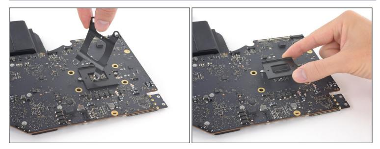
• Lift the heat sink retaining spring and its bracket off the logic board.
