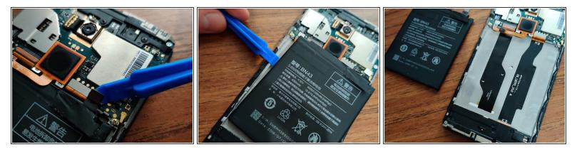
Now we have to remove the battery, luckily the Battery can be removed first after taking the back cover off.
