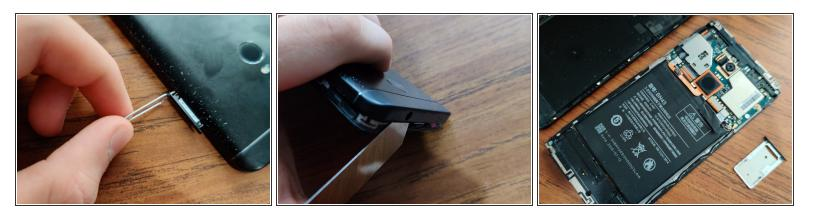
The first thing we have to do is use a pry tool to remove the back cover (make sure to remove the sim tray first)
