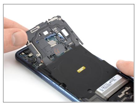
Remove the plastic cover containing the NFC antenna and charging coil.
