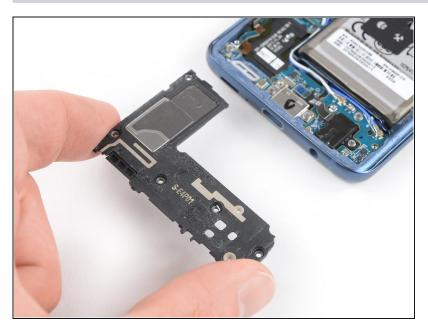
Remove the loudspeaker assembly.
