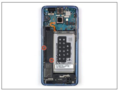
Remove the two 4 mm Phillips #00 screws holding the plastic cover in place.
