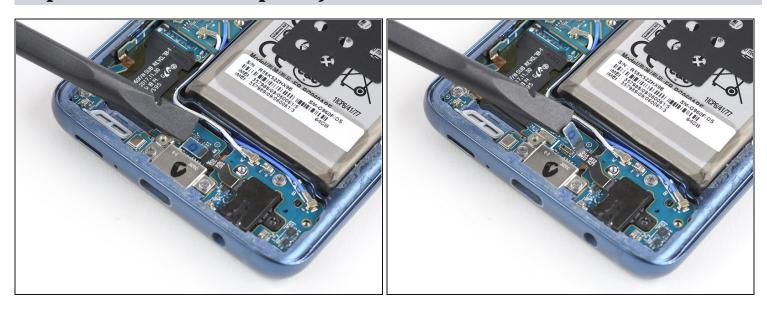
• Use the flat end of a spudger to pry up and disconnect the headphone jack flex cable.
