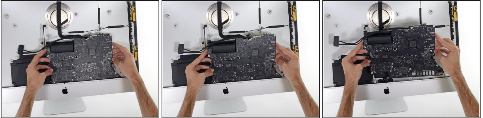
**⚠** When removing and installing the logic board, take care not to damage the delicate microphone ribbon cable at the bottom left of the board.
