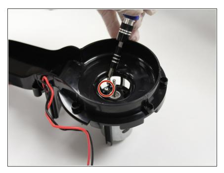
Remove the two 20mm Phillips #1 screws from the bottom of the motor under the fan disc.
