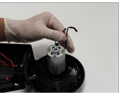
Gently pull the red and black wires from the top of the motor.
