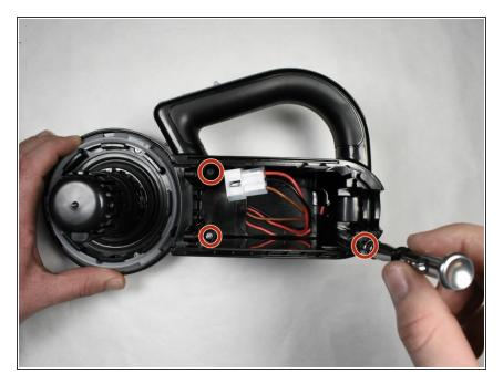
Remove the handle cover by removing the three PH1 20mm screws
