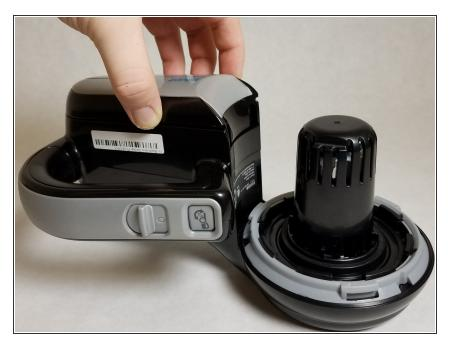
Pull the battery cover up and then slide it away from the motor to remove.
