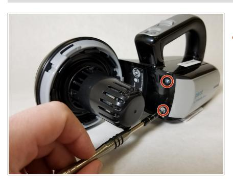
Remove the two 10 mm screws from the motor casing with a Phillips #1 screwdriver.
