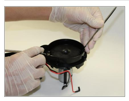
Use a second metal spudger to pry up the fan disc.
