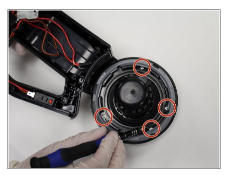
Remove four Phillips #1 screws from the motor housing.
