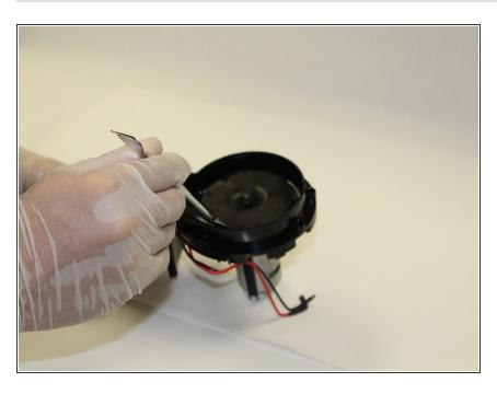
Insert one metal spudger underneath the fan disc located on the opposite side of the motor.
