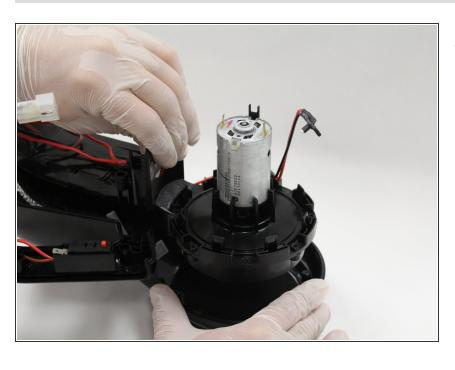
Lift the motor casing from the outer shell of the vacuum by pulling up on the motor casing away from the outer shell.
