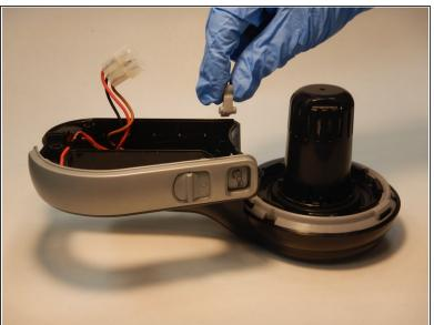
Pull the pivot linkage from the handle.
