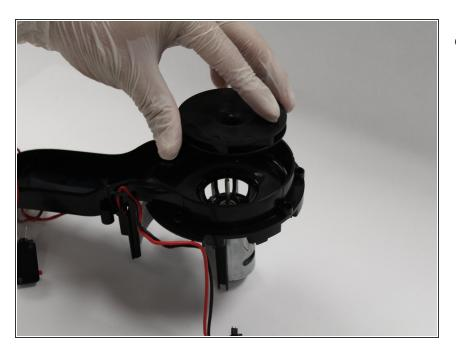
Pull up on the fan disc to reveal the motor screws.
