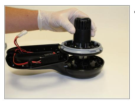
Lift the motor housing straight up to remove it from the rest of the vacuum.
