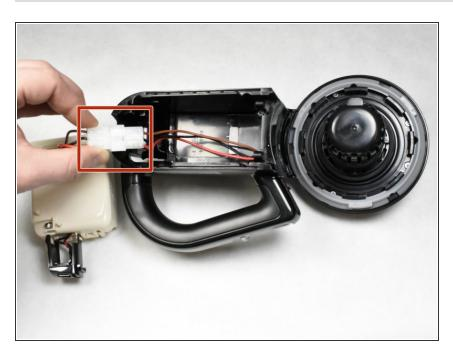
Disconnect the quick connect wire harness that connects the motor and battery located in the battery storage compartment.
