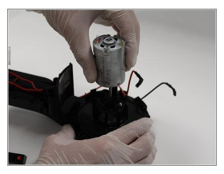
Flip over the motor casing and remove the motor to be replaced.
