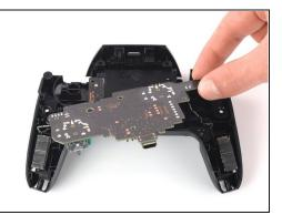
• Lift the motherboard carefully as to not damage the wires and flip it to reveal the backside.
