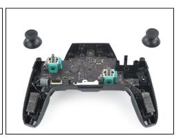
• With light force pull the two joystick caps off of the controller.
