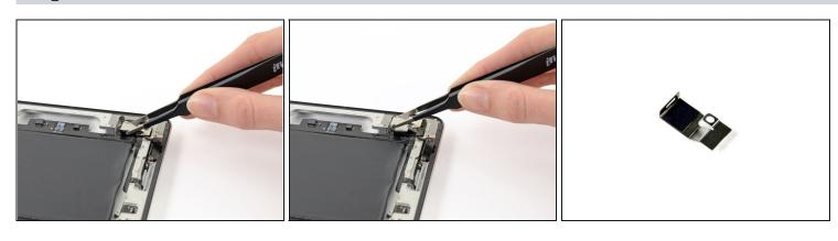
• Lift the rear-facing camera metal retainer clip straight up from its recess in the rear case.
