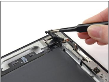
Use a pair of tweezers to remove the rubber cover up off the rear-facing camera housing.
