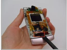
Use a spudger to detach all of the connections to the motherboard in the back of the phone by the screen.
