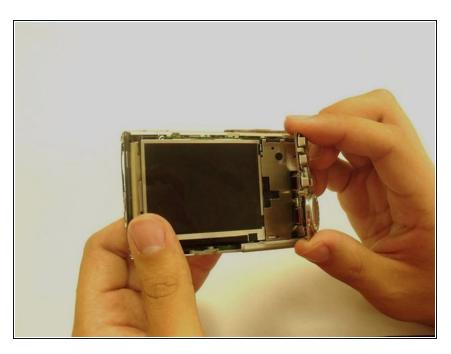
The plate holding the buttons is on the right side of the camera. Use your fingers to open it to the right, away from the LCD screen. Do not twist or force the panel open. It should lift easily.
