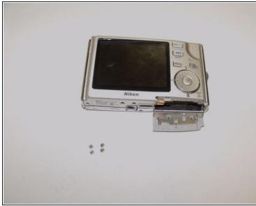
• Remove the four screws adjacent to the SD/battery opening using a Phillips #00 screwdriver.
