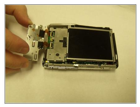
• Pull on ribbon cables to disconnect ribbon cables.
