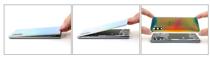
Lift up and remove the back panel.
