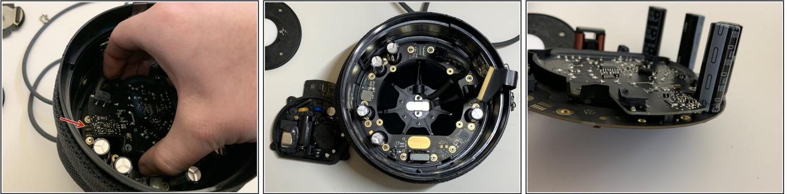
**⚠** Be sure to pull straight up (orange arrow) when removing the power supply (after removing the screws). This connector is fragile and easily damaged during removal and installation!
