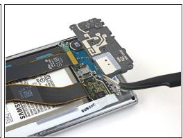
Use a pair of tweezers to remove the loudspeaker.
