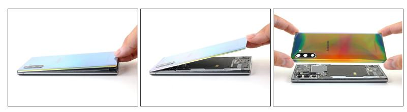
Lift up and remove the back panel.
