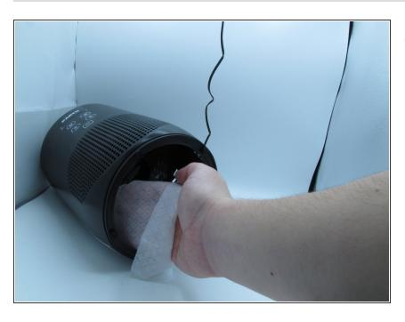
Using a sanitizer wipe, wipe down the inside of the empty filter compartment.
