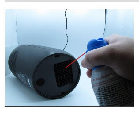
Using the can of compressed air, spray any dust out of the fan compartment. To reassemble the air purifier machine, follow these instructions in reverse order.
