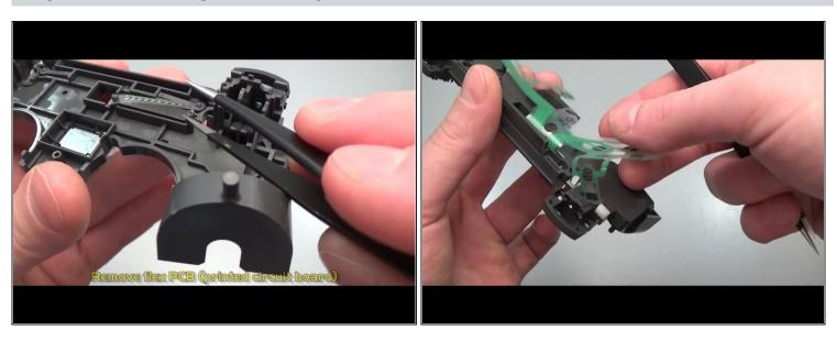
• There's a piece of Mylar with a circuit on it to detect the buttons. Use the tweezers as shown.
