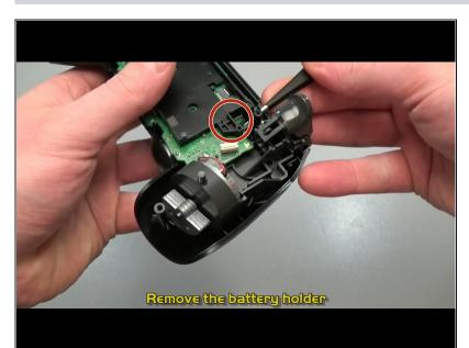
The battery brace is held by friction by pegs on either side of the brace. Use tweezers to remove the brace
