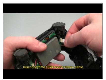
• Undo the interface connecting the ribbon cable to the mainboard.
