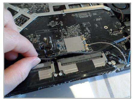
Take a note here how the cable for the left audio speaker (I'm pinching it) is routed loosely above the RAM slots. After you reinstall the logic board, you need to put this back in a similar style.
