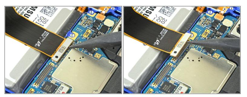
Use the pointed end of a spudger to disconnect the display cable connector from the motherboard.
