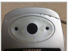
Pry the speaker cover off display, to reveal 2 screws.
