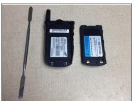
Press on black button next to battery and use metal spuger or other pointy object to pop the battery of the back.
