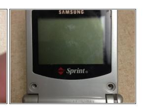
Remove the 2 0.3mm screws from display
