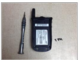
Remove 4 0.6mm screws with a T6 Screwdriver.
