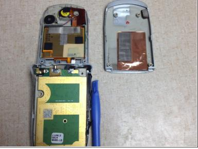
Use a case opening tool and pry the case of the display.
