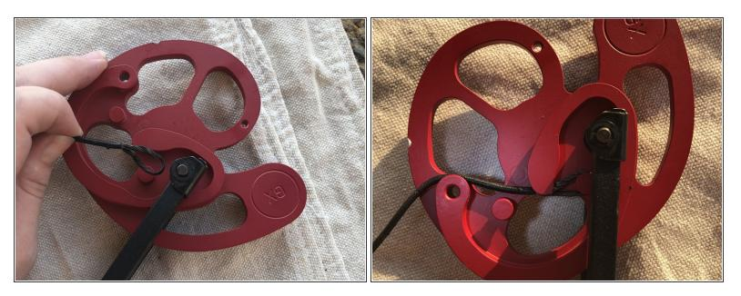
• Spin the cam until the peg is showing on the inside towards the cable rod. Attach the black power cord to the peg. Make sure it is between the pegs when going through the cam as seen below.
