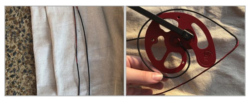
• Find the end with the longest-serving (the black part of your string) of your black and red string. It is the starting side. As seen in the image the top sting is the longest-serving because it does not have red intertwined. Attach it to the cam on the peg and wrap it around the groove between the limbs and feed it through.
