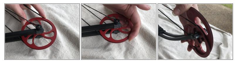
• Check that all the strings are secure in the grooves on the cams. Do this by running your hand along the string making sure it is flat and tight unlike the above image.
