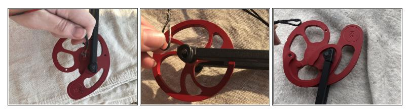
• Unhook the black power cable from both the cam and idler wheel.
