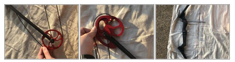
Hook the string to the cam again by putting it between the bow with limbs up, around the idler wheel, under your cable rod, and over the limbs.
