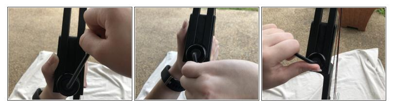
• Tighten both sides of your bow with your Allen wrench with clockwise rotations.
